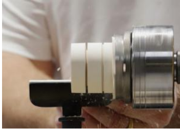
Start with a tenon on the blank
