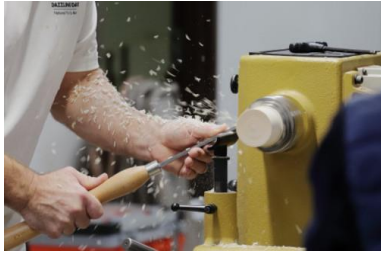
Start with a tenon on the blank
