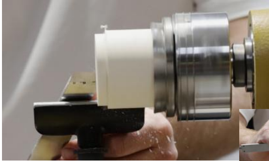
Start with a tenon on the blank
