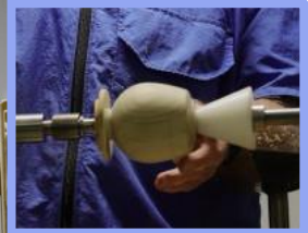
Jig for removing tenon and finishing the bottom
