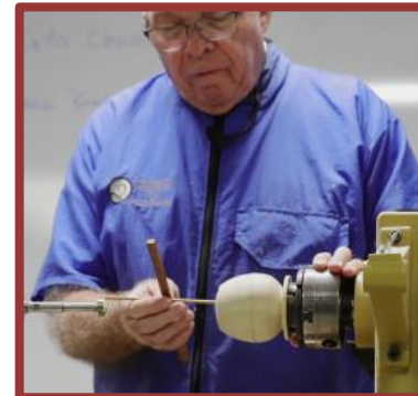
Determining depth and drilling to depth with forstner bit
