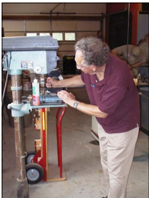
Don Greenheck at the drill Press drilling the Bin Pho tool shaft
