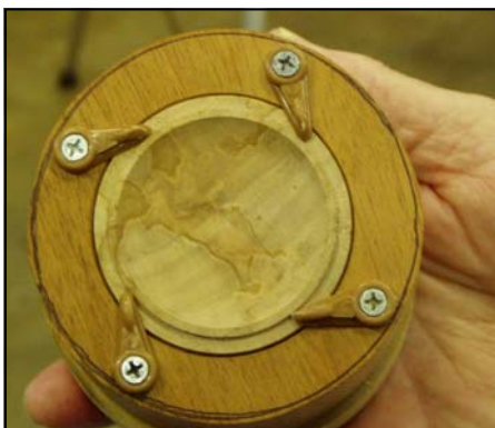
One of the chucking methods shown by Jim Jacobs used to turn the underside of a lid, involved using "clips" usually used to hold panes of glass in cabinets.
