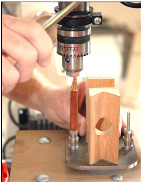
Brad added this jig to a bench-top drill press to convert it to a pen assembly tool. The pen tip is being pressed into the turned blank in this photo.
