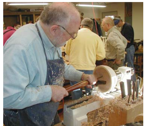
David Winter cleaned up the interior finish of his bowl with his favorite 1/2" thick scraper.
