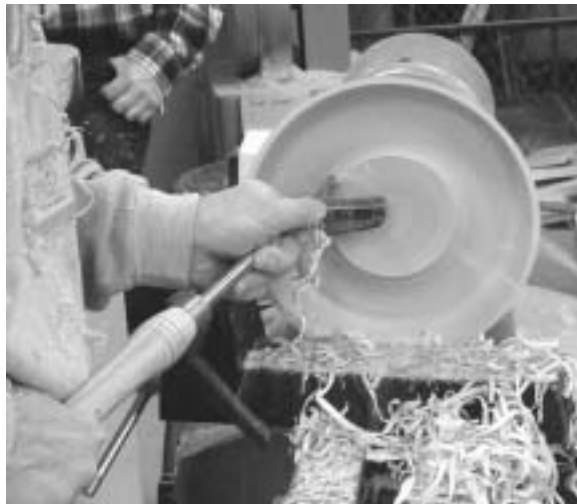
Top left - After shaping the exterior of the bowl, Wayne started turning a tenon to clamp in the scroll chuck prior to hollowing the bowl's inside.
