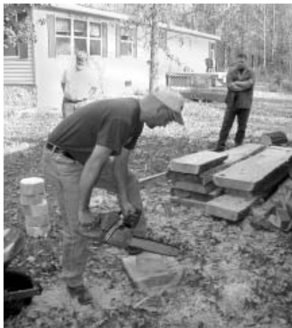
Right - Todd Schweim demonstrated how he rough shapes bowl blanks with a chain saw. A local saw mill cuts the four-inch slabs from trees cut in the area. He can get six to eight bowls from each slab.
