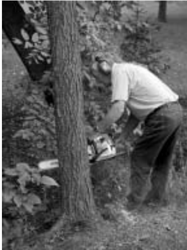
Above left - John made the notch cut on the back side of this elm tree in the direction he wanted the tree to fall.
