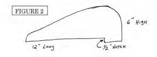
Another simple jig from Jim is a feather-board made from ¾" pine lumber. The feather-board will keep the workpiece snug against the fence when ripping lumber on your table saw. It can be used along with the push-stick shown above.
