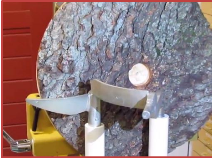
OneWay coring set-up for a natural edge bowl
