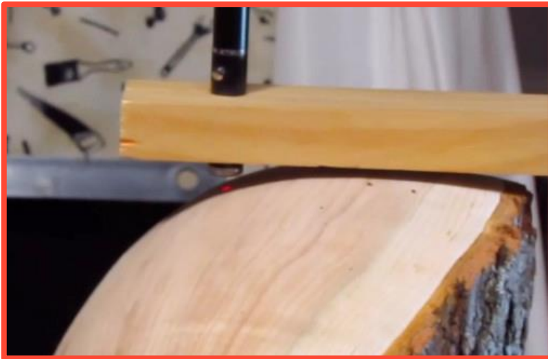
The laser dot on the outside of the bowl
