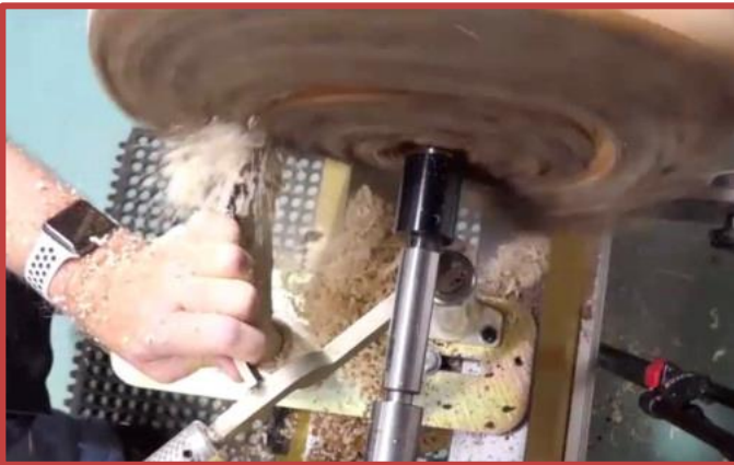
Coring and the core pops out
